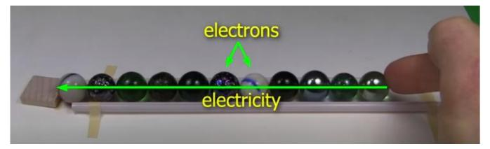
The atoms in the wire are crammed together cheek to jowl, which, while it makes the going slow, also has the electrons more or less abutting one another. When the switch is turned on, a force is created to move the electrons, with each pushing its neighbor, which in turn pushes its neighbor and so on all the way through the wire.
